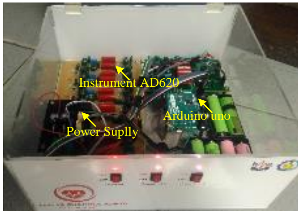
Figure 9. The result of 12-channel ECG design with AD620
